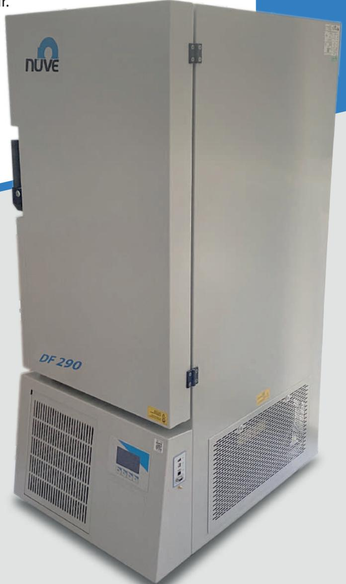
Unlike traditional deep freezers with cooling coils located outside the cell, the DF series deep freezers utilize the DirectFREEZE™ technology, where the cooling coils are placed underneath the shelves. This enables direct heat transfer to the samples placed on the shelves, resulting in more efficient results compared to the heat transfer provided by air in conventional systems.
