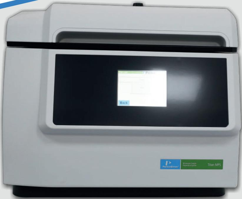
Microwave digestion is used to dissolve bound metals in a sample matrix in a liquid. The sample is digested by subjecting it to strong acid in a closed vessel and increasing temperature and pressure through microwave irradiation. Once heavy metals are dissolved, their quantity can be determined using elemental techniques.
